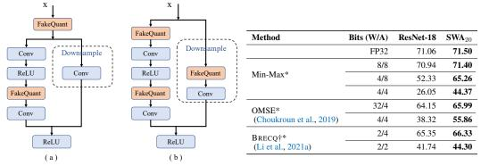
Figure 7: Different ways of inserting activation quantization nodes. Our method obeys the left side one while AdaQuant adopts the right side one.
